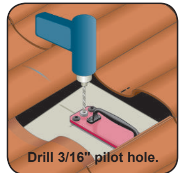
Step 4: Seal the initial tile nail hole. Using a 3/16" drill bit and drill guide (FJ-Drill), drill pilot hole along the rafter center.
