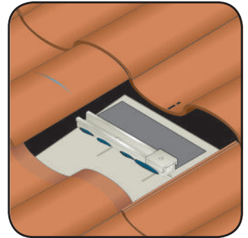
Step 8: Install subflashing and seal as needed if double flash is desired.
