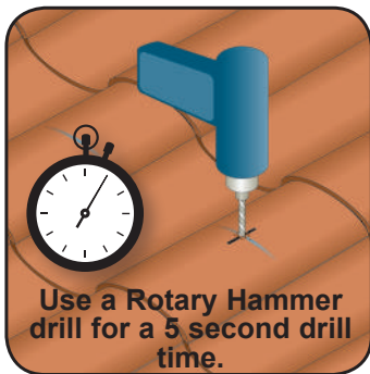
Step 10: Using a 1/2" carbide drill bit and ROTARY HAMMER DRILL in hammer mode, drill through the tile. See online video at www.prosolar.com for details.
