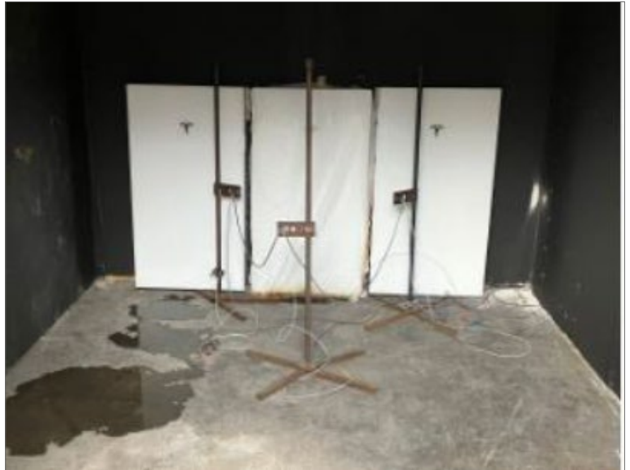
Figure 10: Photo 6 from the Test Report Displaying “Cheesecloth as is After the Test”
